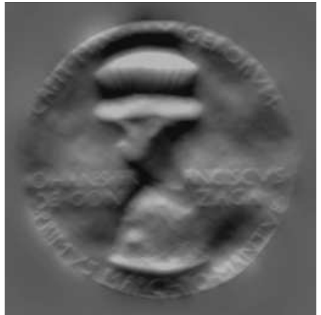
Figure 14: (a) Image input for linear shape-from-shading analysis using steerable image transform. (Steering was used to accommodate different light directions). (b) Resulting range map, displayed as a low-resolution 3-D plot. (c) Same range map, with pixel intensity showing surface height. This simple mechanism, using biologically plausible filters, correctly derived the image surface characteristics.
