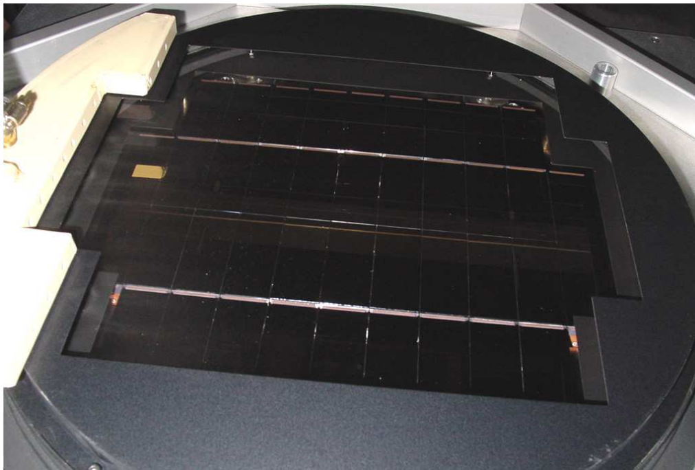
Figure 1. The mosaic of CCDs seen through the entrance windows of the cryostat of MEGACAM, on its testbench at CEA.
